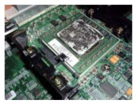
3. Push the lever back down and fix a processor.
